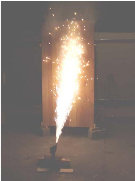
**Figure 4-14a. Gerb impinging on wood panel.**
